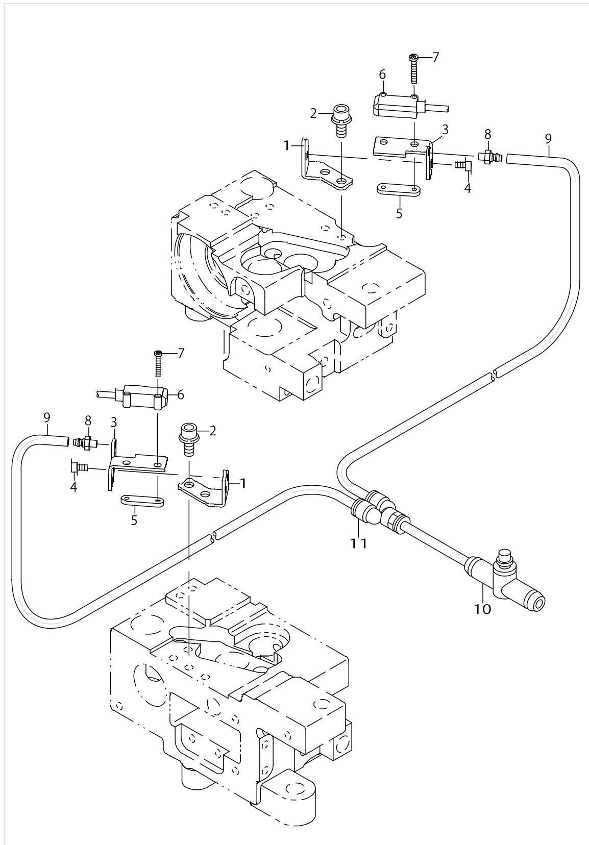
BOBBIN THREAD DETECTING COMPONENTS
