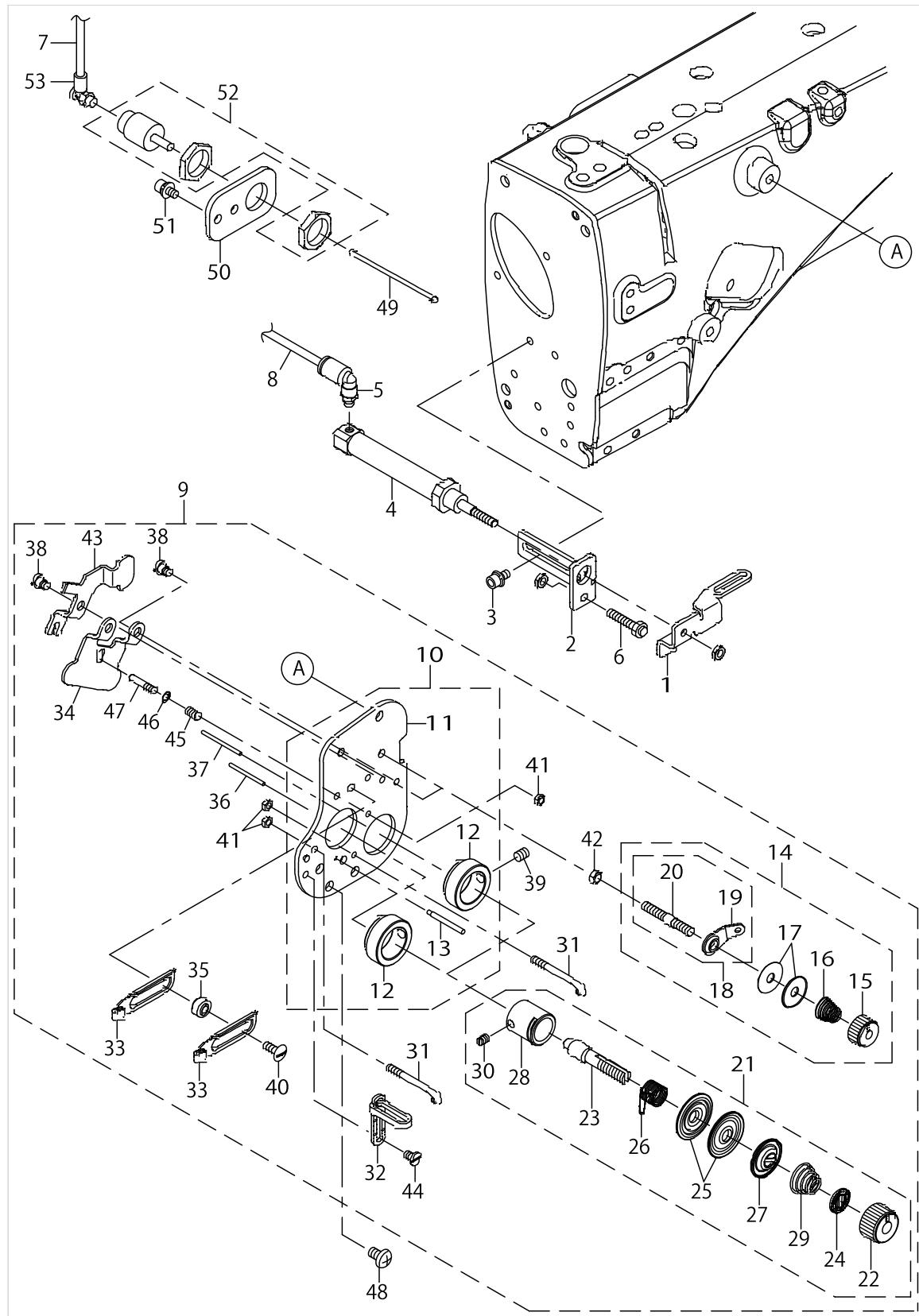
THREAD TENSION & WIPER COMPONENTS
