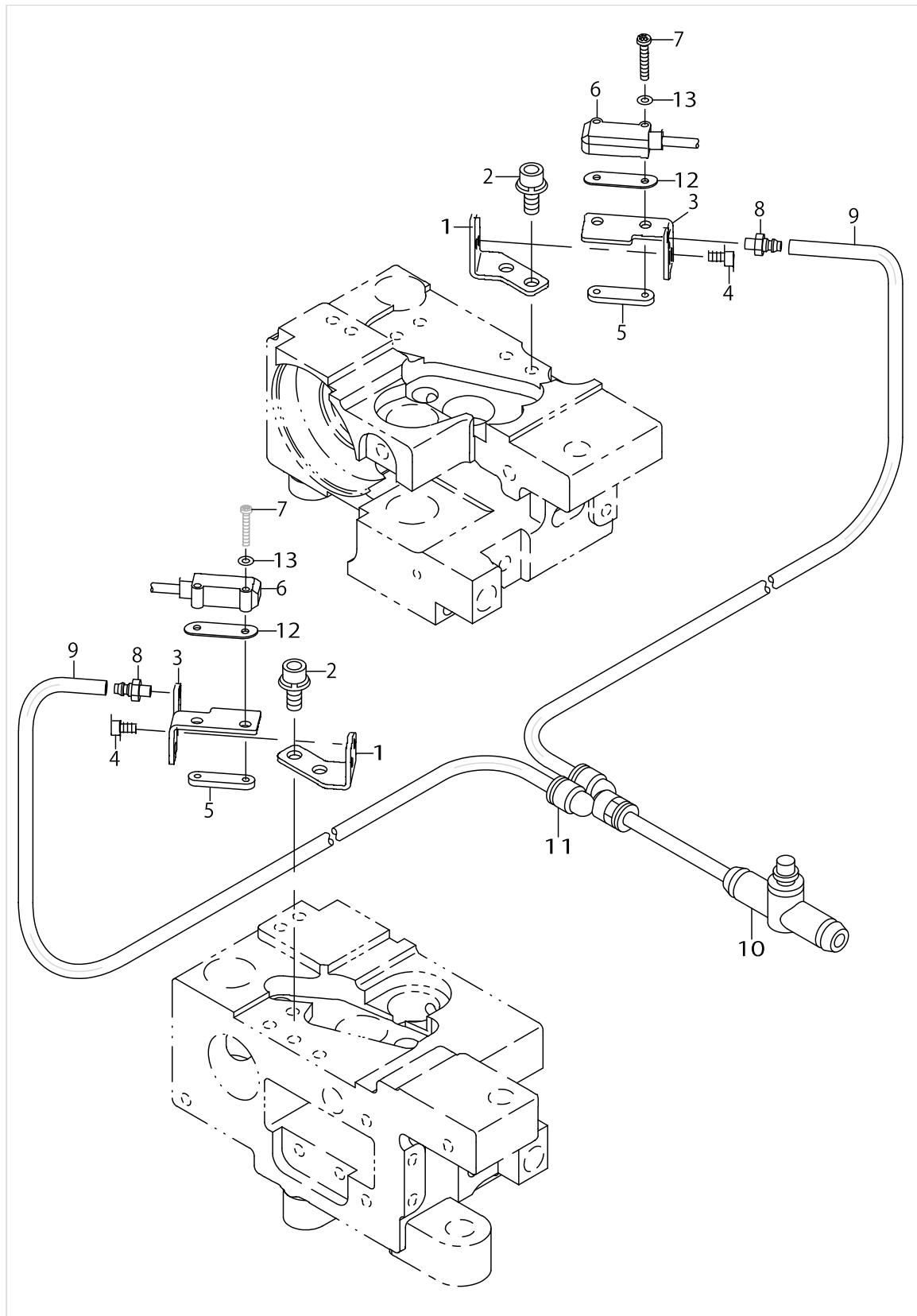
BOBBIN THREAD DETECTING COMPONENTS
