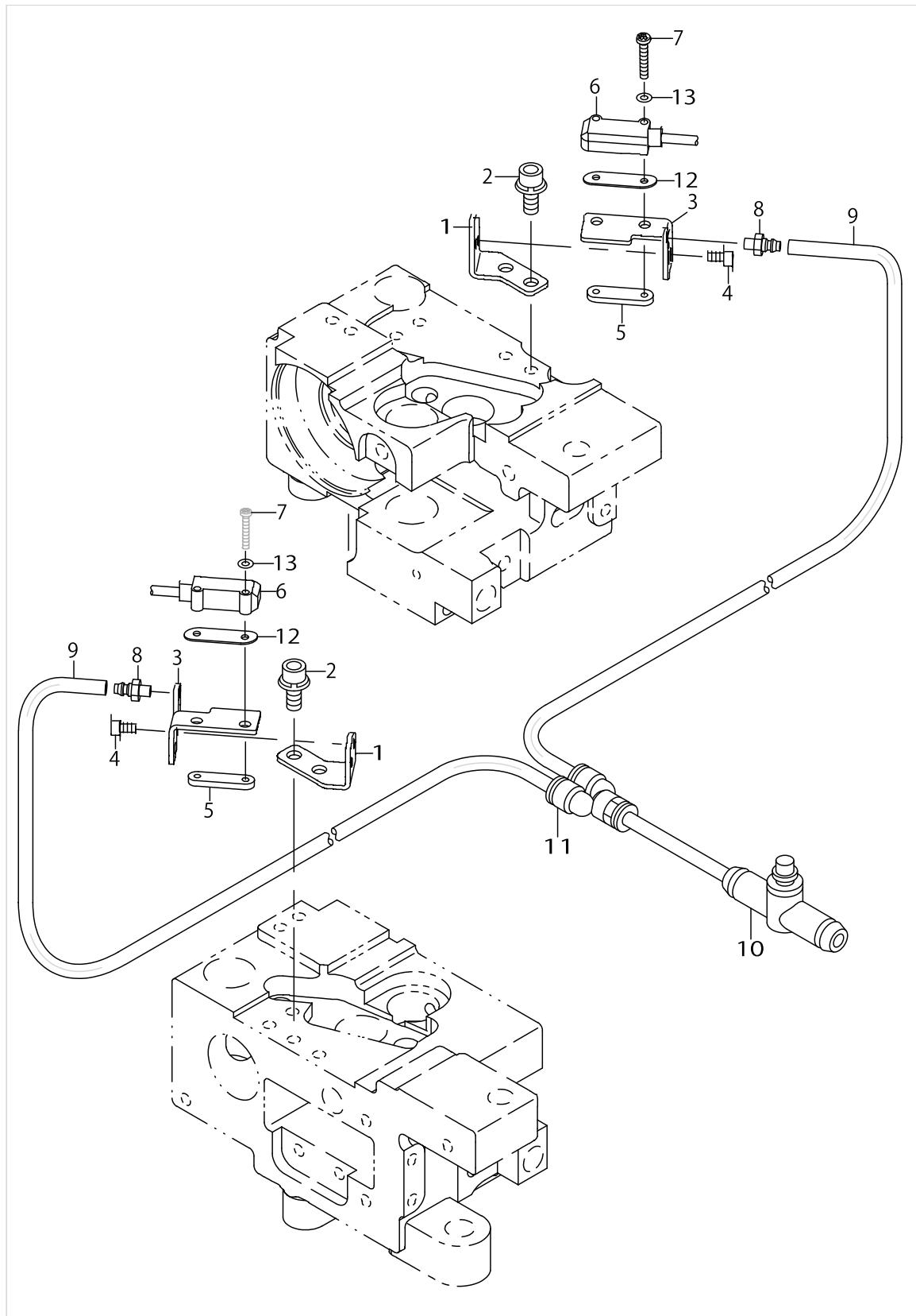
BOBBIN THREAD DETECTING COMPONENTS
