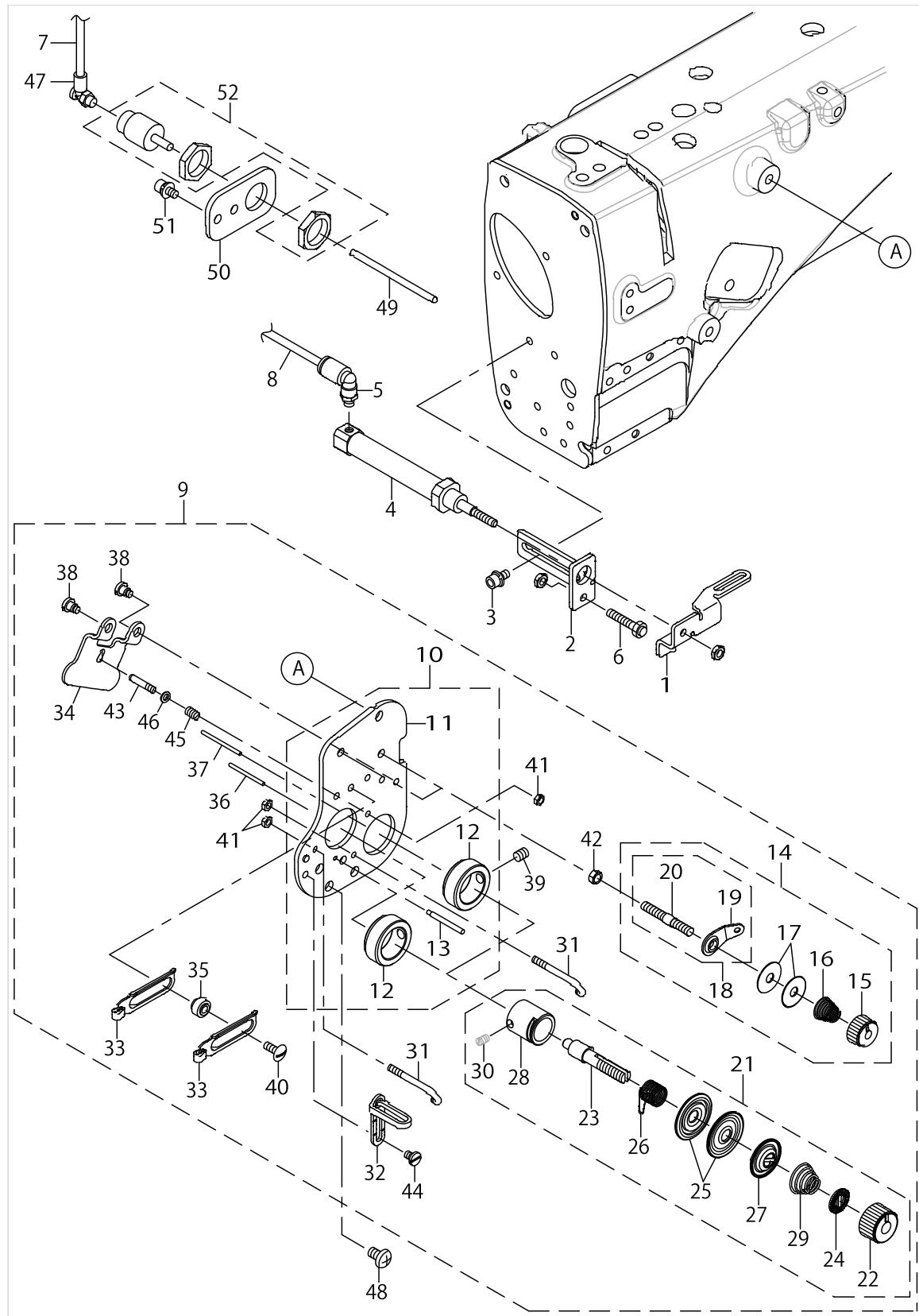
THREAD TENSION & WIPER COMPONENTS
