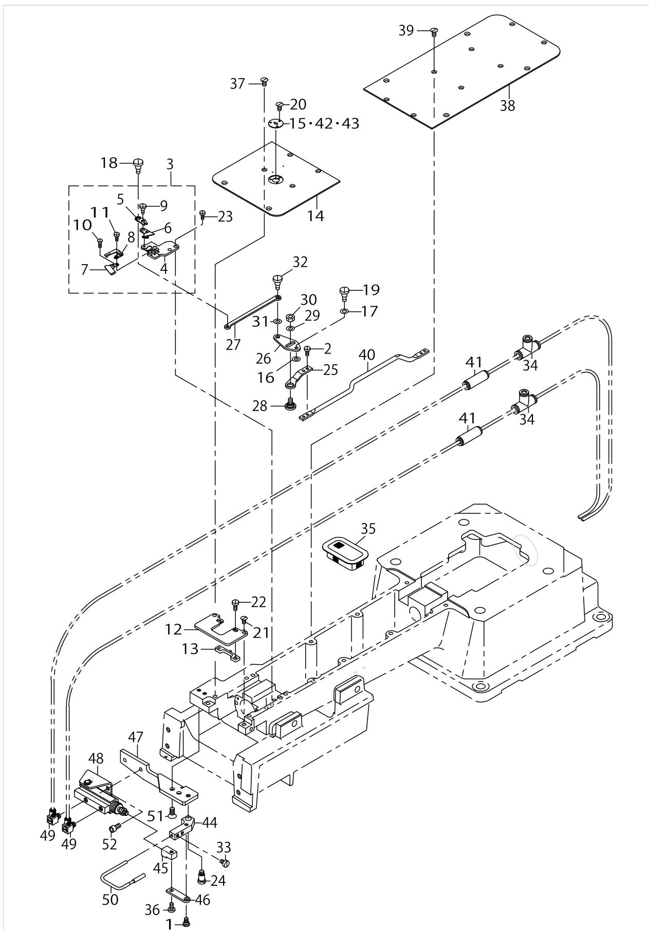
THREAD TRIMMER MECHANISM COMPONENTS (1)
