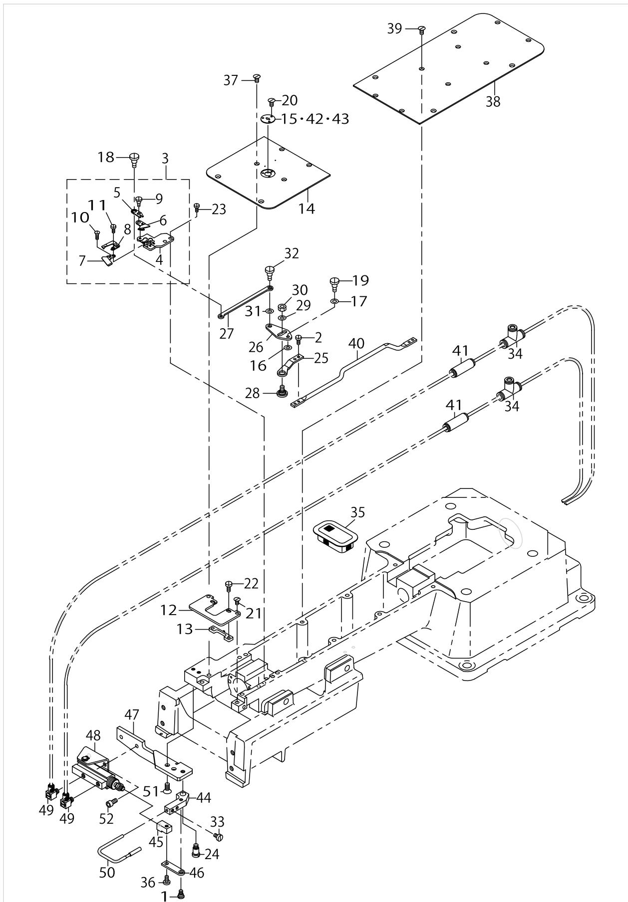
THREAD TRIMMER MECHANISM COMPONENTS (1)
