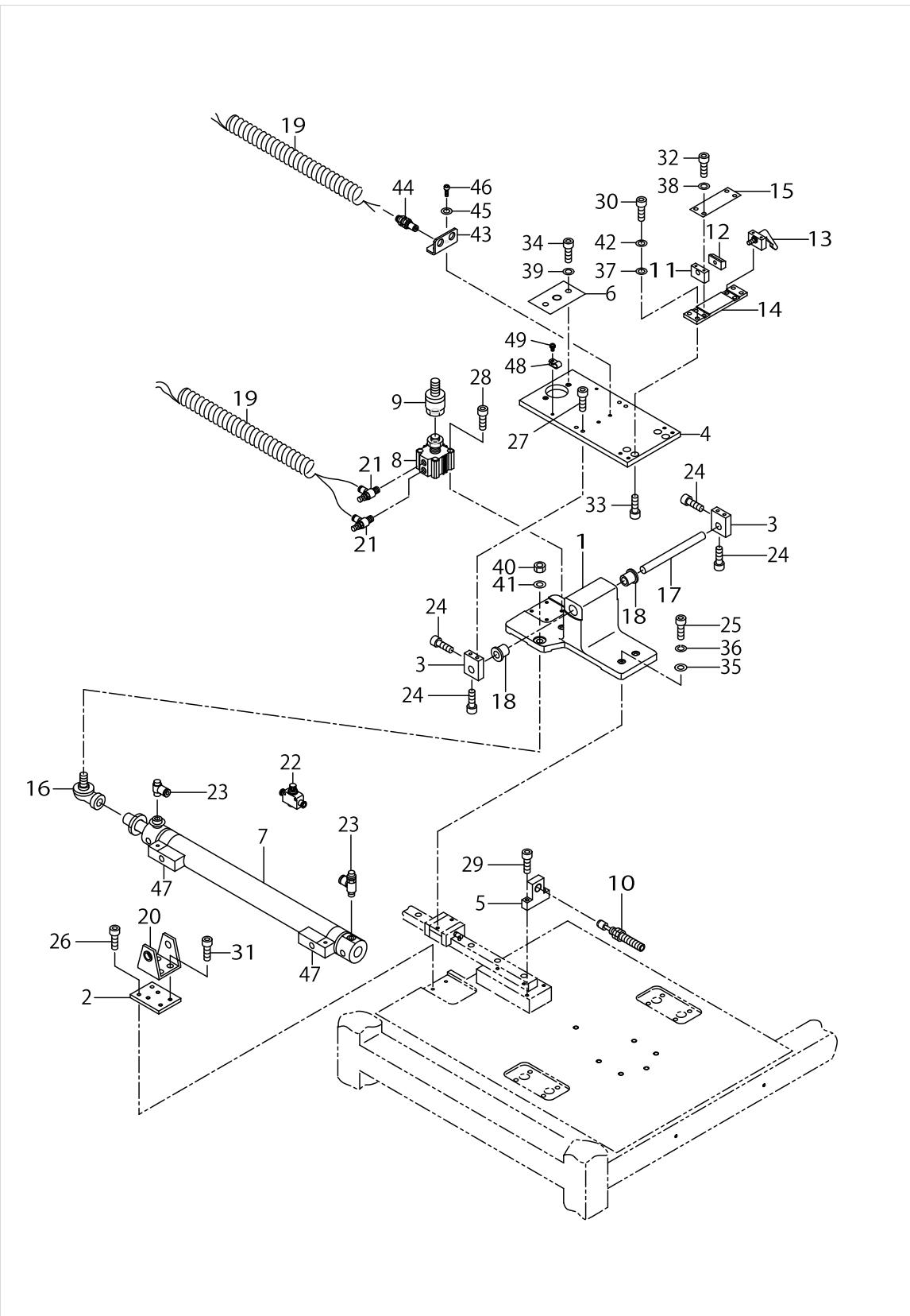
FORM PLATE MECHANISM COMPONENTS
