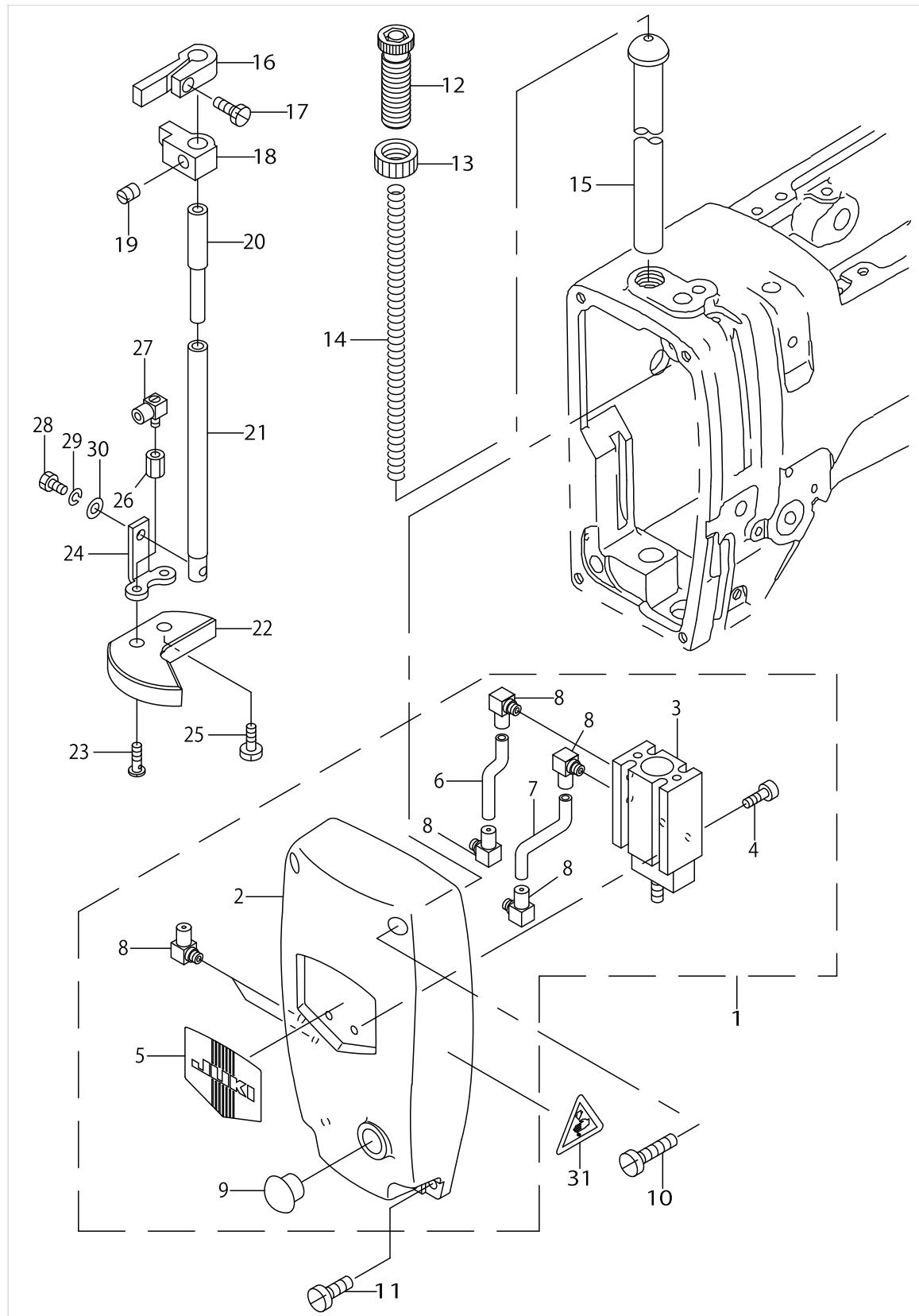
PRESSER MECHANISM COMPONENTS
