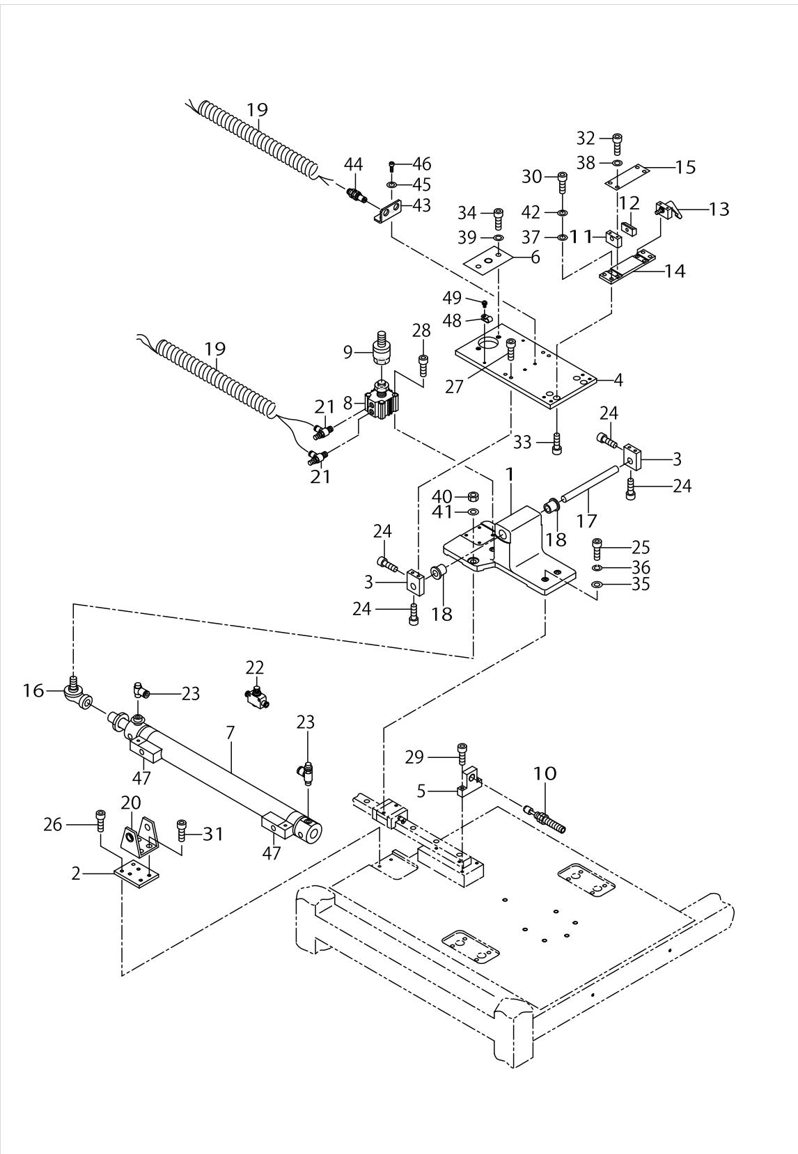
FORM PLATE MECHANISM COMPONENTS
