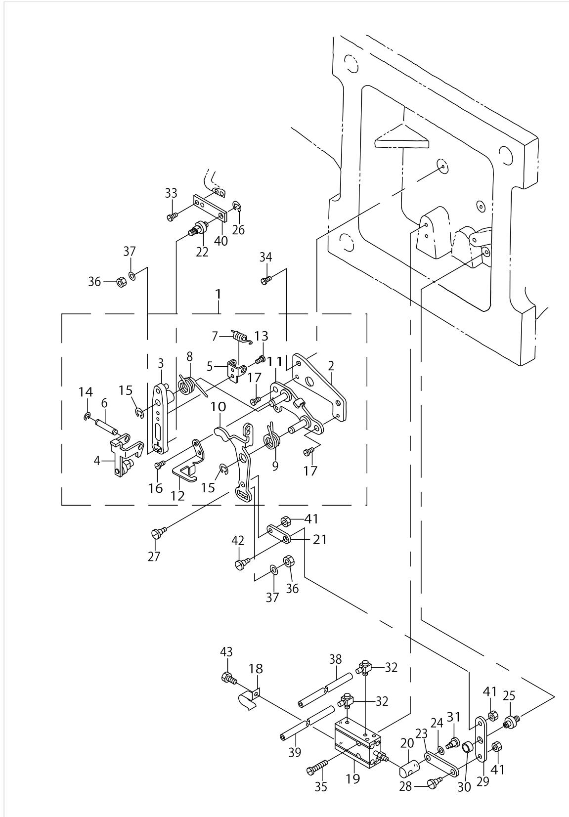
THREAD TRIMMER MECHANISM COMPONENTS (2)
