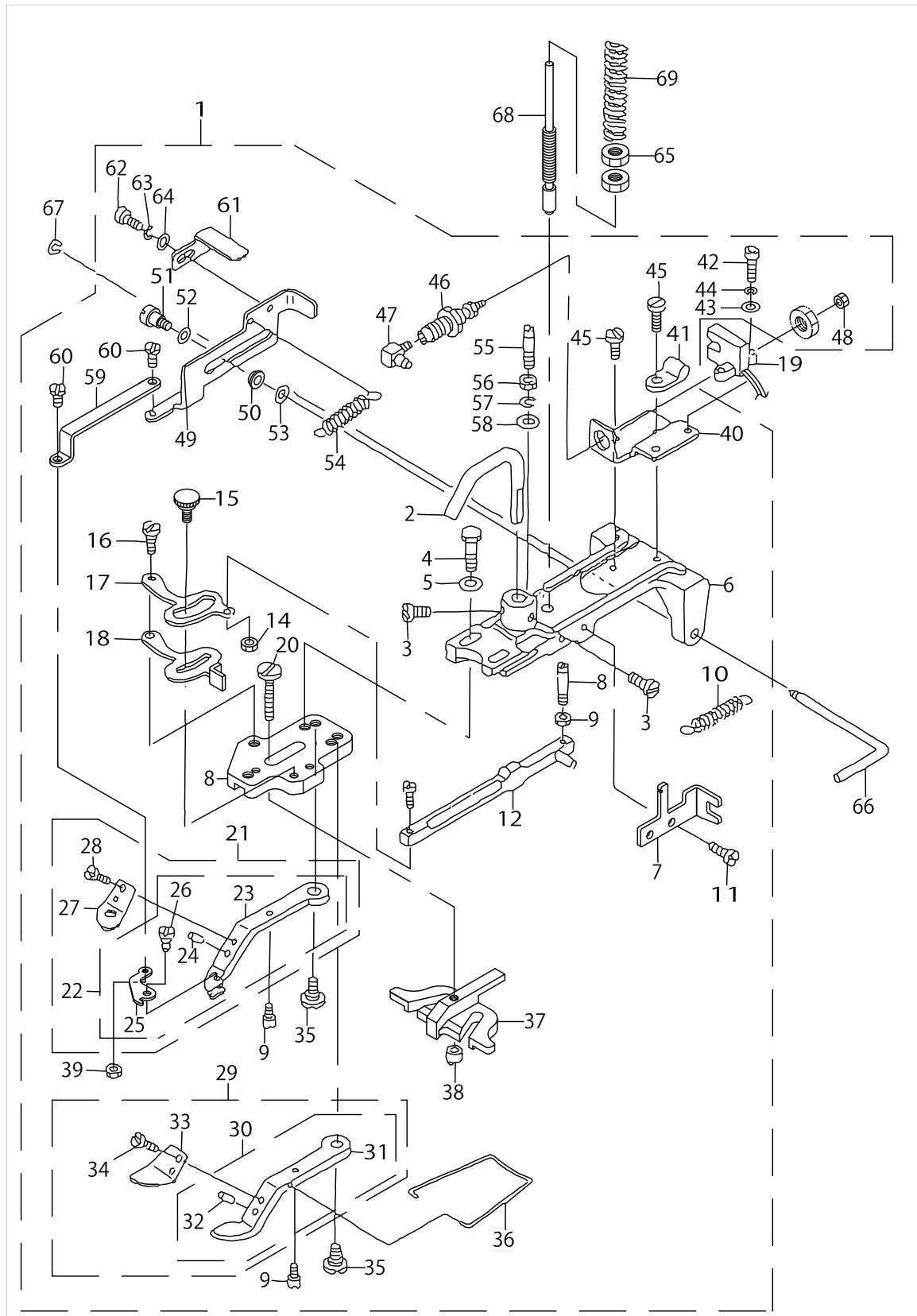
FEEDER CLAMP MACHANISM COMPONENTS
