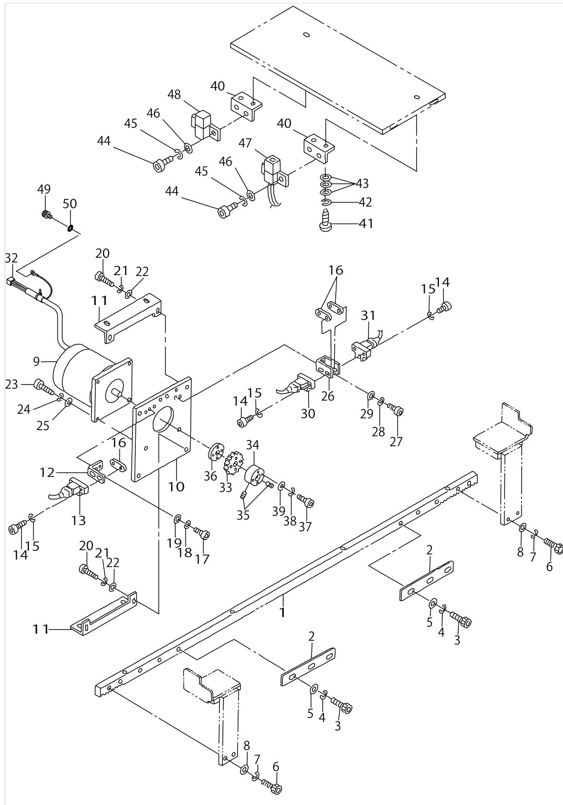
FEED MECHANISM DRIVE & SWITCH COMPONENTS
