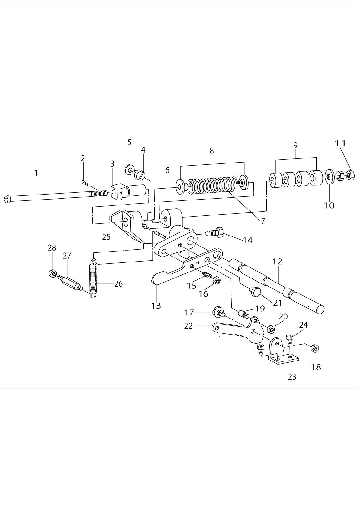
STOP MOTION MECHANISM COMPONENTS
