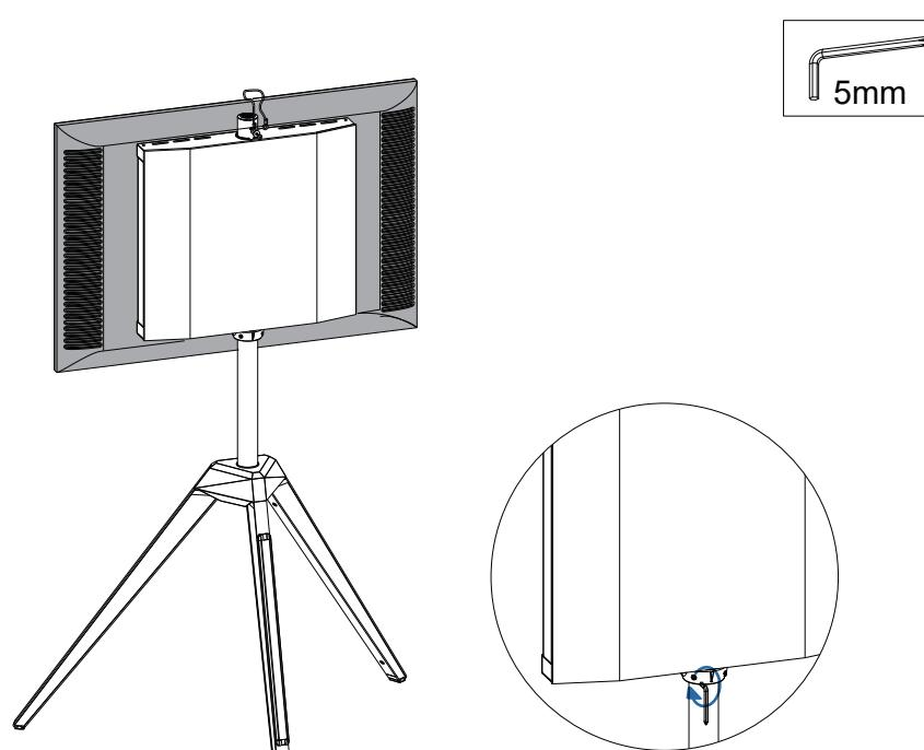
**EN** Use a 6mm Allen wrench to adjust the TV backplane to a proper height.
