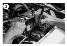
Label each of the factory relays accordingly, using a marker or label printer before removing them from the cover.
