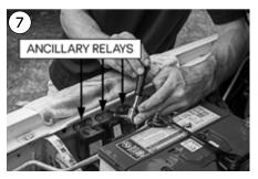
In most cases the factory ancillary relays in this location will need be relocated in order to mount the auxiliary panel and relocate the factory accessory relays.
