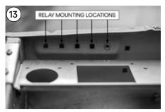
Recommended alternate mounting locations for the factory relays. To mount the relays M6 nutserts may need to be installed at these locations - Refer to the 'Nutsert Installation' page.
