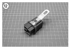
As pictured, ensure the fold in the bracket is facing away from the relay. This relay is now ready to be installed\*
