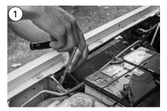
Remove 4× bolts from the factory relay cover. If applicable, set aside any aircon hardline clips/clamps.
