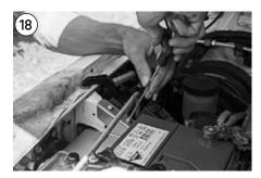
Fix the aux panel in position to body using the supplied M6X16 SS Allen bolts, M6 flat washers, and M6 serrated flange nuts, Include any aircon hardline clips/clamps set aside in earlier steps.
