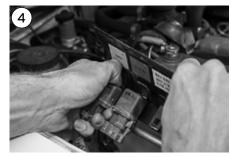
Remove all of the relays from the underside of the cover by carefully sliding them off the mounting tabs, then set them aside for later steps.
