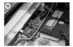
Note: It is recommended that the factory aircon line is mounted using rubber lined P-clamps (not supplied), or is very gently manipulated away from anywhere that might contact. Cover with conduit if necessary.
