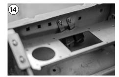
Relays may need to be installed at angle to allow enough slack in the factory wiring harness. If enough slack cannot be achieved, the harness sheathing may need to be manipulated to allow for further movement.
