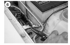
Remove 4× factory screw-grommets from the cover's original mounting points. This is achieved by compressing the fins on each grommet whilst levering it out of it's hole.
