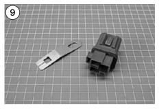
Supplied relocation bracket and factory Nissan relay. At this step remove any protecting film and or residue from the bracket using thinners or isopropyl alcohol.
