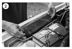
Tilt the factory relay cover towards the start battery to expose the relays on the underside.
