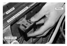
Note: The new mounting location may vary depending on the year model of your vehicle. We have chosen to mount the relays on the inner guard closer to the firewall. Drilling additional mounting holes may also be required. Alterna-
