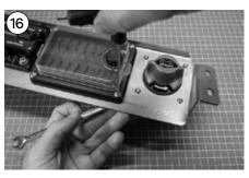
At this step mount any electrical components to the aux panel. Make sure to leave any protective film on the panel intact until all works have been carried out to prevent marking.
