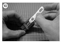
Fit the relay bracket to the relay by sliding the tab end of the bracket into the channel on the back side of the relay until seated.
