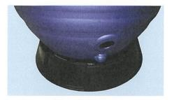
Before filling tank with sand, place nub on bottom of tank into notched out piece of the base, twist to the right till snug.
