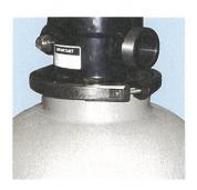
Make sure that the screws of the clamp are lined up with the seams of the tank. Tighten two screws on clamp a little at a time. Alternating from side to side so that both sides are tightened equally. Failure to follow these instructions will result in a leak at the clamp.
