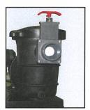
Thread one of the slide valves on to the front threaded opening of the dual port pump. Prior to doing this you will need to wrap Teflon tape around the male threads of the slide valve. Give to slide valve approximately 8-12 wraps – clockwiseover the threads. This will eliminate leak in the future.
