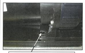
Figure 7 - Plastic pump housing mount
