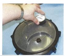
Figure 25b — Installing pressure gauge
