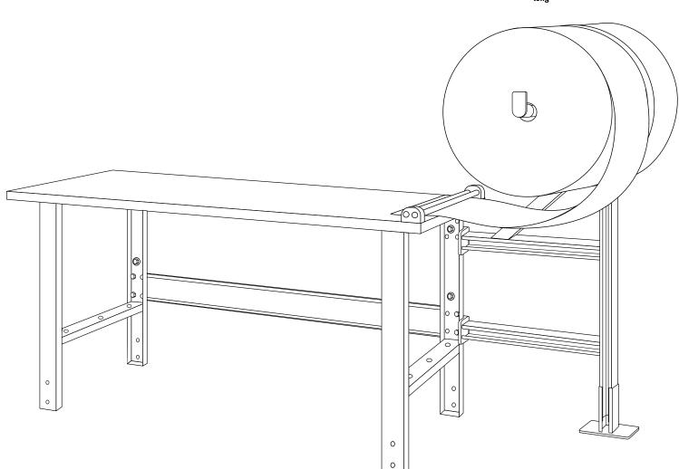
ASSEMBLY OF A SIDE MOUNT SPOOL HOLDER TO 3500 SERIES LEG. Need to talk to you about this assembly.
