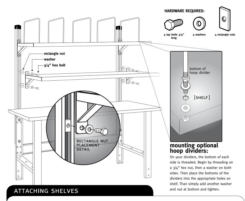
**step 1:** Assembly of Carton Shelf should be done once the overhead uprights are in place and fastened to bench legs. Begin by assembling hardware supplied for the shelf (shown above) which consists of four 3/4" hex bolts, four washers and four rectangle nuts per shelf.
