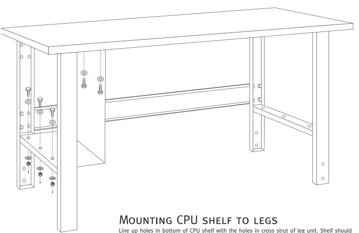
be at center of strut front to back. Attach shelf to leg using tap bolts, washers and hex nuts. Position shelf so that it is parallel to leg unit, straight up and down. Mark holes from top of shelf to underside of worksurface. Drill 1/4" pilot holes, then use lagscrews and washers to fasten cpu shelf to worksurface.
