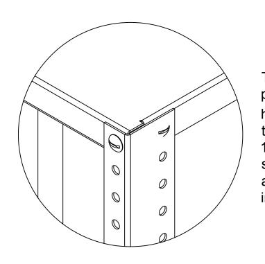
The figure to the left shows the position of the uprights. The top has the first hole starting  $\frac{1}{2}$ " from the edge, the bottom hole starts 1" from the bottom edge. The side faces of the uprights are 2" and the front/back faces are 1" in width.
