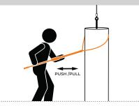
Capture and control a suspended vertical object around its circumference
