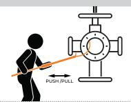
Control a suspended load by threading the cable through a secure attachment point
