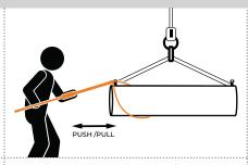
Capture and control a suspended horizontal object around its circumference
