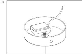
Cut the excess cable of.
