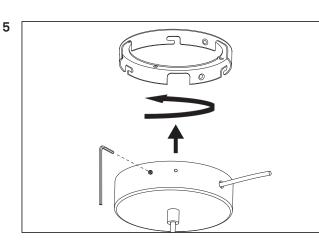
Attach the ceiling plate to the top plate by turning the ceiling plate.
