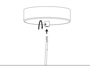
Lead the fabric cable in through the cable relief at the bottom of the ceiling plate. Adjust the cable to the desired length.
