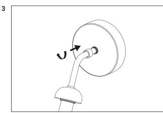
Mount the cover plate by hand threading the fastener until it is tight.
