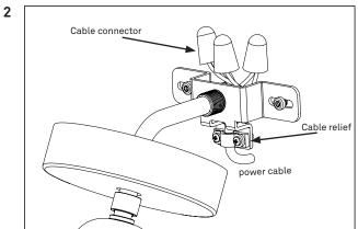
If the power cable is surface mounted make sure to put the cable through the hole in the cover plate before the following,
