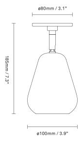
**Anoli Spot Recessed** is designed for mounting to a ceiling or wall for a seamless finish. An excellent choice when space is at a premium, it delivers bright task light from its adjustable arm.
