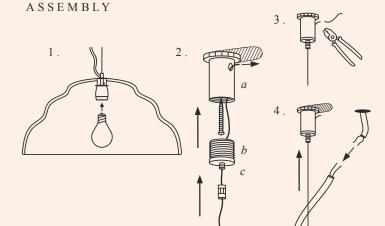
The installation must be performed by an authorised electrician. *Please make sure the electricity is turned off before installation.*
