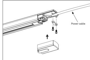
Connect the power cable to the cable terminals. Match the brown wire with "L", the blue wire with "N" and the green/ yellow wire with the grounding symbol.
