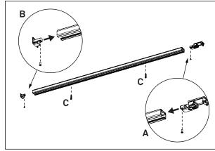
A: Slide the connector module in one end of the track. Lock it in place by tightening the screw.
