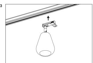
Insert the adaptor on to the desired position in the track.
