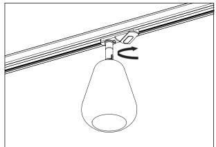
Lock the lamp in place by turning lock to the center position.
