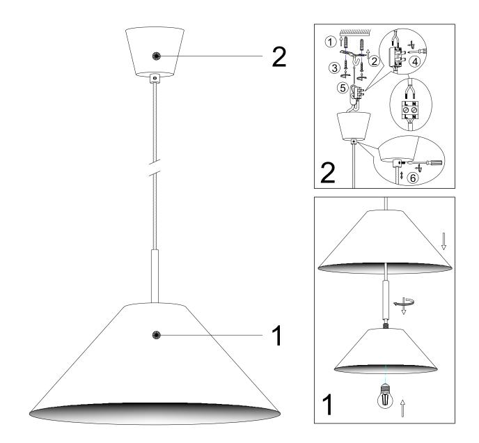
1, Make sure power is off on the outlet , before the installation.
