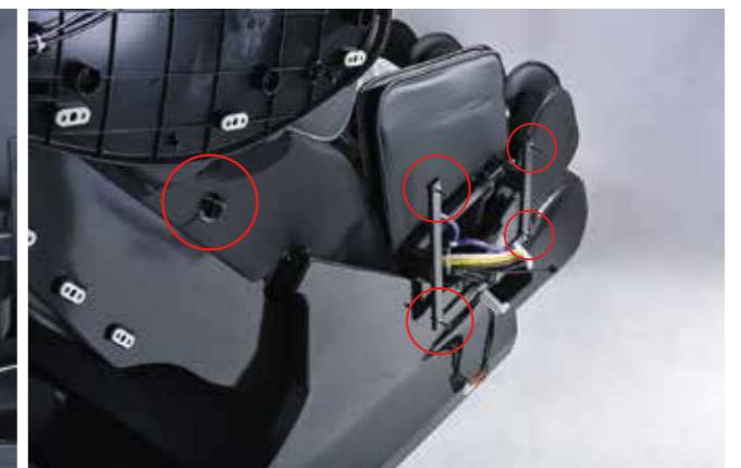
Here is what it will look like once you have fastened in the double-threaded screws.
