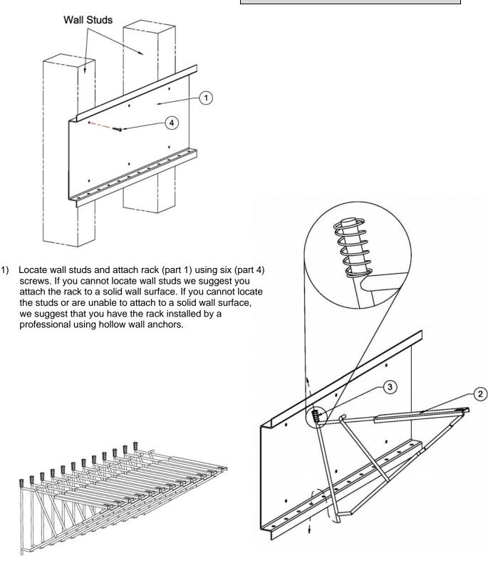
2) Guide hangers (part 2) with springs (part 3) into the top of the upper frame assembly as shown in diagram. Push upper end with spring into upper hole and then insert lower part of hanger into bottom hole of rack.
