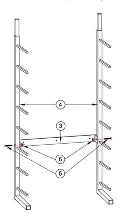
2) Attach wall brace (part 3) to upper tube rails (part 2) using bolts (part 5) with hex nuts (part 6).
