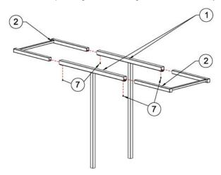
4) Slide upper frames into lower frames. Adjust to size of clamp being used and insert two pcs M6X8 set screws into lower tube assembly and tighten with Allen key.(part 9).
