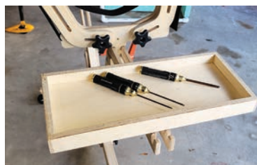
The optional tool tray is handy for keeping frequently used tools handy while working on projects.
