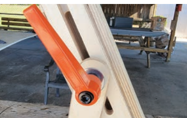
These ratcheting handles make securely tightening the stand very easy on the hands.
