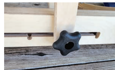
A great addition to the floor stands are these "lock in" notches that enhance the weight bearing capacity of the stand without needing to add more material.
