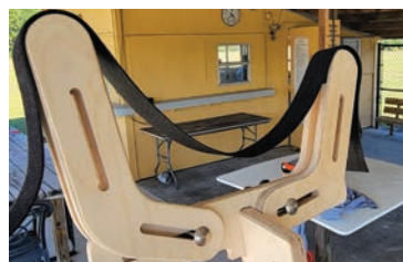
Velcro straps allow models to be cradled without putting their weight on the wood parts.
