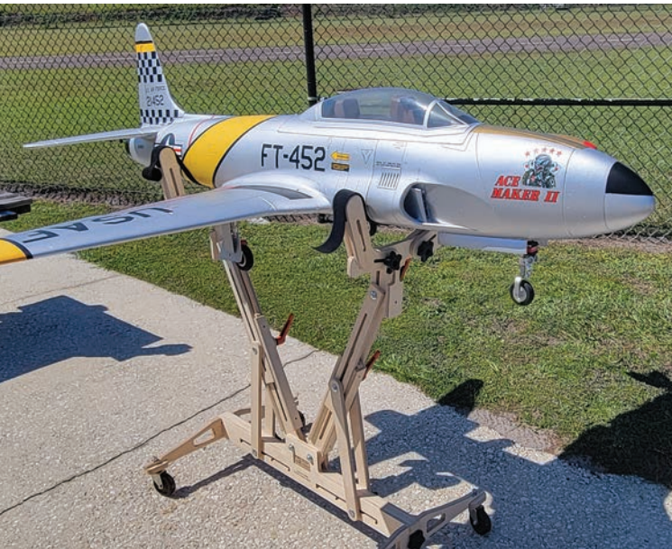
Shown with the HSD T-33, the floor stand easily supports this heavy foam jet without damaging the delicate foam.
