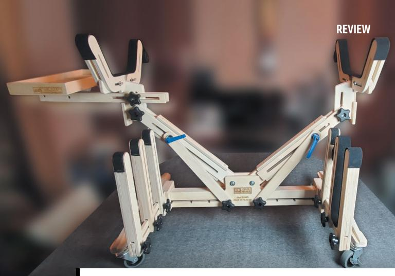
The stand assembles quickly and is recommended for aircraft in the 10cc to 120cc range, weighing up to 60 pounds.
