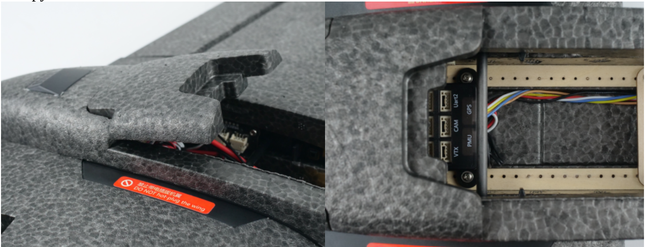
ad. Slide the smaller rear canopy towards the rear of the fuselage and ensure no wire between the canopy and the carbon rod.
