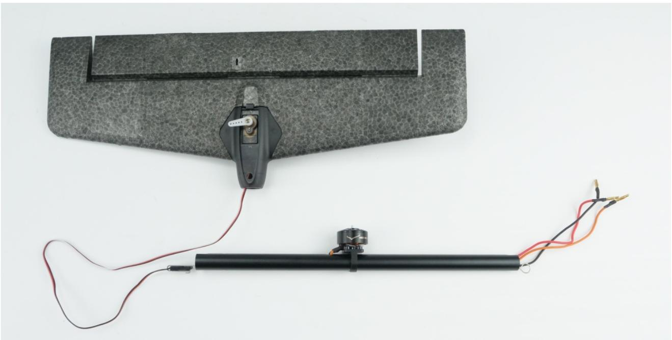
Tips : using the U shape of the wire and clip it onto the servo connector
