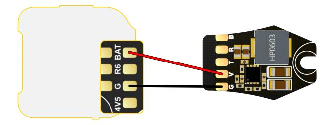
The red wire should be soldered to the BAT pad of the flight controller or the positive pole of the power cable, with an input voltage range of 2-6S lithium battery.
