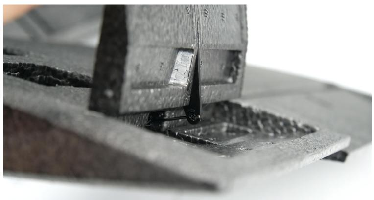
6. Apply glue to the side walls as shown for ease of removal when needed in the future
