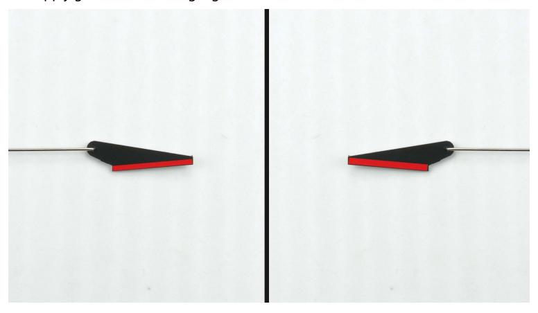
4. Slot the steel linkage into the opening beneath the split flap
