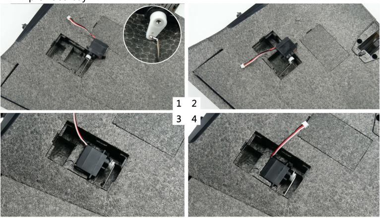
8. Slot the servo wire into electronics bay II and connect to the flap connector found inside. Then repeat on the other wing.
