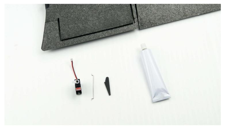
2. Slot the steel linkage into the control horn
