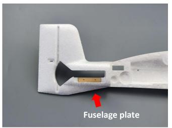
Bond the wooden plate and fuselage quick-release mounting base
