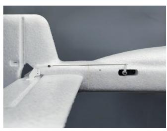
Note: When installing the horn linkage, power on the servo and set to the neutral position.
