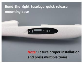
Note: Ensure proper installation and press multiple times during adhesion, press as needed to avoid improper adhesion.
