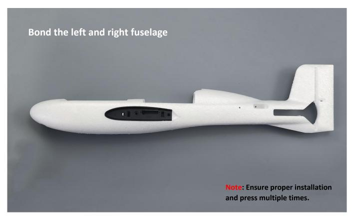
Note: Ensure proper installation and press multiple times during adhesion, press as needed to avoid improper adhesion.
