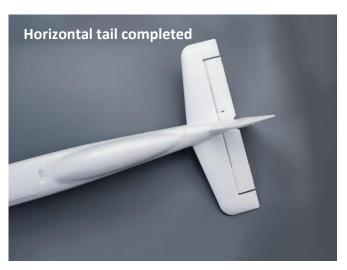
Note: Ensure proper installation and repress during adhesion, press as needed to avoid improper adhesion.
