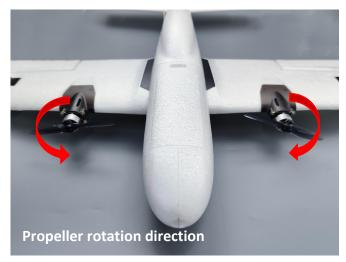
Note: Before installing the propeller, ensure the correct motor rotation direction.
