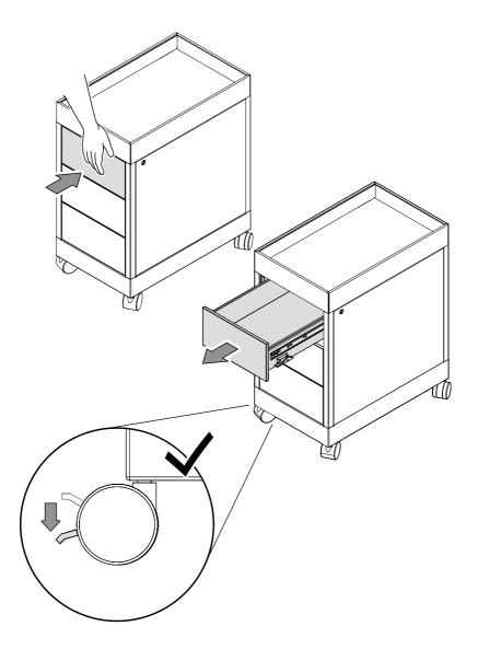
Please note that the trolley has a lock to prevent tipping, which only allows you to open one drawer at a time.
