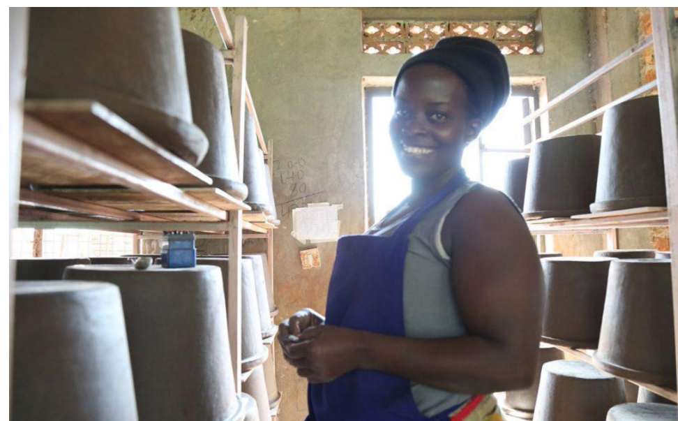
Above: Local Ugandan employee of Spouts (from whom we purchase the ceramic water filters for our Clean Water Project) tends to the filters' production process. The filters are made of local clay and sawdust, and remove more than 99% of contaminants that cause water-borne illnesses.
