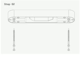
Fix the ceiling rose canopy to the ceiling using 5mm wood screws. Fixings are not provide. Note: Be sure the screws sit within the counter sink
