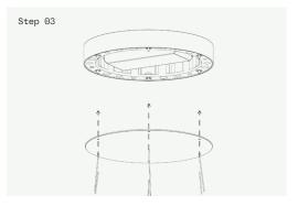
Feed the suspension cables through the cover plate. Start with the first cable and work your way clockwise. Be careful not to tangle the cables.
