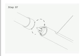
Screw the glass diffuser to the main body of the light to finish installation.
