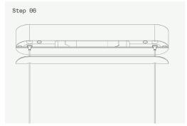
Cover the ceiling rose canopy with the two half's of the cover plates. Be careful not to let the cover-plates touch any part of the wires or cable grips, this could cause the light to short.
