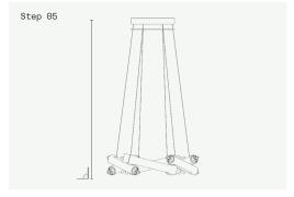
Set the light to you desired height making sure the light is level. You can do this by pulling through and realising the suspension cable through the cable grips.
