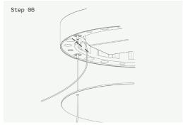
Once the desired position has been met neatly trim the excess cable with a pair of knipex. When all cables have been cut carefully slide the cover plate over the cables and fix to canopy. Do not let the cover plate touch any part of the cable grips, this could cause the light to short.
