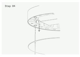
Feed the suspension cables through the cable grips. Do this by pushing the nipple on the cable grip in, then feed the cable though and out the side of the grip. Realising the nipple of the cable grip holds the cable fixing in place.
