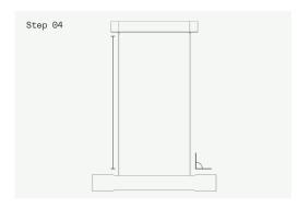
Set the light to you desired height making sure the light is level. You can do this by pulling through and realising the suspension cable through the cable grips.
