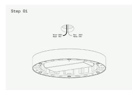
Wire the driver to the mains via the terminal blocks in the driver, making sure they connect to power in.
