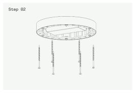
Fix the ceiling rose canopy to the ceiling using 5mm wood screws. Fixings are not provide.
