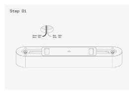
Wire the driver to the mains via the terminal blocks in the driver, making sure they connect to power in. Note: Align ceiling void hole to driver access point.
