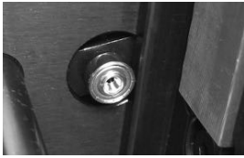
Adjustable guide bearing (2015-2018) next to moving die holder.
