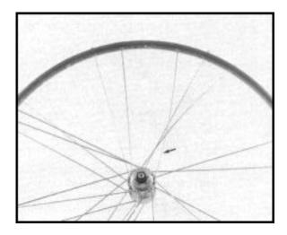
Back on the original flange, a spoke from the third group crosses above two spokes from the inside of the flange, then passes under the next inside spoke for a 3-cross pattern.
