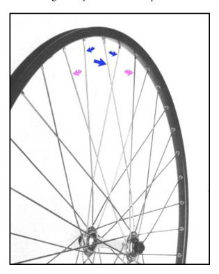
An example of tension balancing: If this right-side spoke needs to pull the rim to the right, but it's already too tight and creating a "low" spot, loosen the spoke and its 2 neighbors from the left side (blue arrows) and tighten the 2 nearest spokes on the right side (red arrows).
