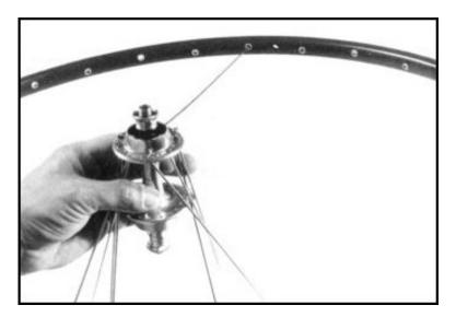
For the common "left. handed" rim, the first spoke of the first group (the No. 1 spoke) is placed in the first spoke hole to the left of the valve hole.
