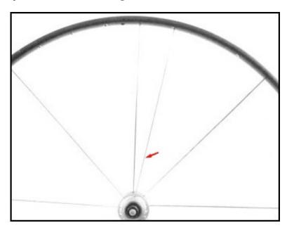
With the wheel flipped over, the first spoke of the second group is placed in the hub just to the right of the No. 1 spoke, which is in the bottom flange. The spoke is placed in the rim in the first spoke hole to the right of the No. 1 spoke.
