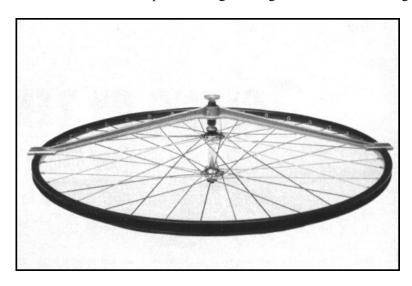
When both ends and the middle of the dishing gauge touch evenly on each side of the wheel, the rim is correctly centered.
