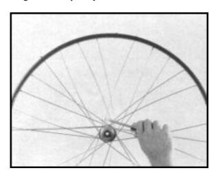
Use a screwdriver to seat inside spokes and gently bend outside spokes to conform to the hub flange.
