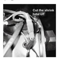
**Step four:** Un-wrap the disconnect the big yellow plug (XT-60)
