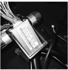
Push the controller into the box. Make sure the charging wire does not get smashed.
