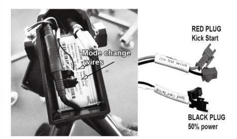
To locate the wires, we wrapped the wires with a white tube and zip-tied the group together. The words 'Zero Start Switch"-KSM, and "Speed Limit" 50%-100% power are on each set of the wires. See pic above.
