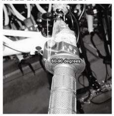
Attach the handlebars as shown. There are 4 screws to assemble or remove the handlebar. The Power S/W should be at a 60-90 degree angle, pointing straight up. This allows the small riders to twist
