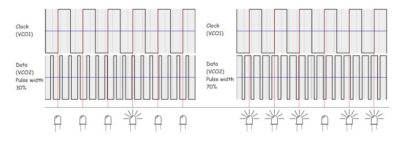
The voltages from the 8 LEDs are then mixed together with different strengths, to create semi-random stepped Voltages. With the Order switch, you can select which part of the LEDs has the strongest influence. This gives different patterns of the voltages generated.
