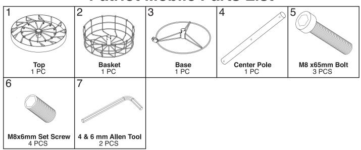
**Materials:** Powder Coated Steel Basket, HDG Steel Center, Powder Coated Steel Base, SS304 Chain Connections, HDG Steel Chains
