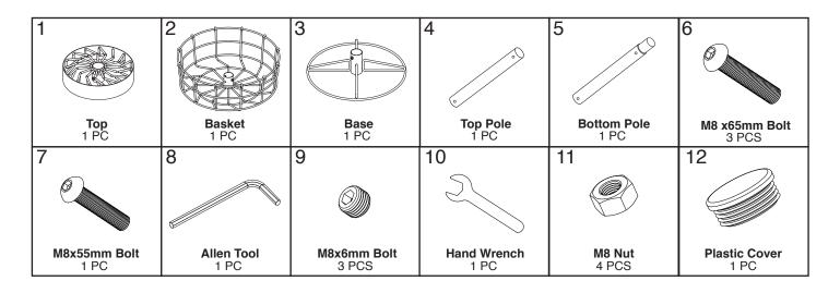
**Materials:** Powder Coated Steel Basket, HDG Steel Center Pole, Powder Coated Steel Base, Zinc Plated Steel Chains
