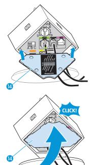
Connecting the base station to the mains power supply
