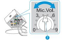
The microphone volume control **7** only adjusts the microphone sensitivity in Phone mode.
