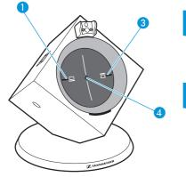
You can also establish or disconnect the wireless link by pressing the PC button (1) or the PHONE button (3) on the base station (depending on the selected mode (PC or Phone), see page 28).
