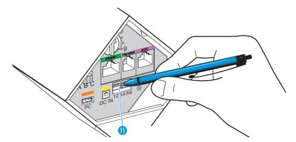
Use a pointed object (e.g. a pen) to set the DIP switches to the desired position.
