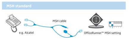
If your telephone has a built-in electronic hook switch supporting the MSH standard:
