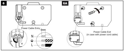
4. Fix the Main unit to Wall mounting bracket
