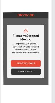
If for some reason the printer stops printing, the dryer will sense this and after giving the user time to fix the issue, it will abort the current operation if filament movement does not resume. Drying will also automatically stop once printing is finished.
