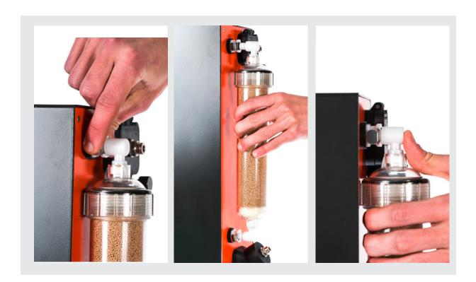
You are done with the desiccant cartridge replacement and can proceed with normal drying operation.
