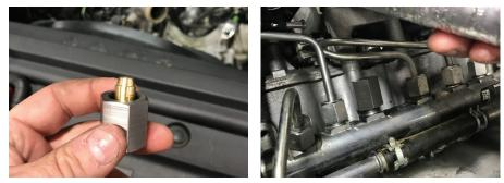
With the CP4 removed from the truck, you can now proceed to remove the gear from the CP4 to reuse on the CP3.
