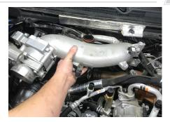
Remove the plastic elbow that connects to the turbo, then continue to remove the EGR system from the vehicle if still equipped.
