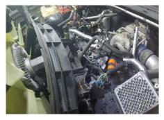
Remove the belt tensioner and the alternator in order to gain access to the front mounting belts of the CP4.
