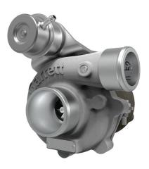
G arrett Boost | Club Line turbochargers are engineered for small engine displacements including powersports, personal watercraft, and automobiles. These turbochargers feature internally wastegated turbine housings and journal bearing rotating groups. Forged, fully-machined compressor wheels can support from 200 up to 350 horsepower for engine displacements ranging from 0.4L up to 2.5L.
