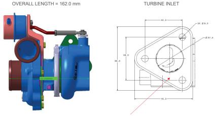
Turbine housing inlet can be machined to V-band with OD of 2.24" (57mm) for use with 1.75" tubing.
