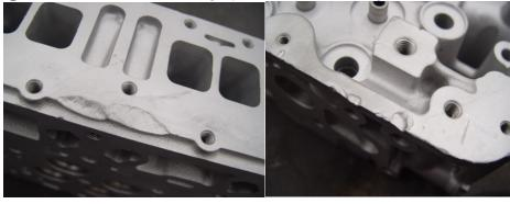
**6** Heads showing signs of electrolysis will not receive core credit.
