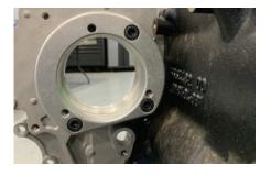
Install CP3 injection pump through the front cover adapter. Pump will need to be rotated towards the driver's fender and then rotated towards the engine block to clear the boss on the block and align the pump mounting holes. Install supplied m8x1.25x40 cap head bolts, lock washers, and flat washers. Hand tighten them in a star pattern until snug, then torque them 33 lb ft
