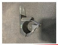
Remove engine harness holder that is attached to the engine harness.
