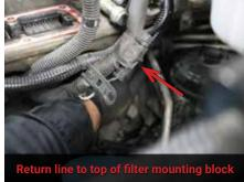
Install supplied banjo fitting to the return port on the CP3 re-using the bolt and sealing washer previously removed. Install previously removed straight quick connect into supplied shorter fuel feed line and clamp. Install quick connect to the factory CP3.
