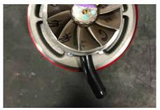
Put turbine housing to center section V-band on turbine housing. Remove compressor housing, install S400 center section into the turbine housing and tighten clamp to 130 IN-LB. With a rubber mallet tap on the V-band, loosen V-band and repeat two more times. After tapping on the V-band a final time double check the clamp torque. Spin turbocharger shaft while pushing up, down, and side to side to ensure turbine wheel doesn't contact turbine housing.
