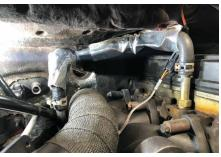
Using the factory exhaust housing to exhaust elbow V-band clamp attach hot pipe but leave it a little bit loose so you can still move it. Take the two exhaust manifold bolts that you removed earlier and start through the hot pipe mount. Tighten the V-band clamp, then torque the two exhaust manifold bolts to 35 Ft-Lb.
