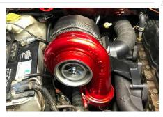
section V-band to 120 IN-LB and gently tap with a rubber mallet to seat clamp. Loosen clamp and repeat two more times. After tapping on clamp for the final time double check torque. Tighten intermediate charge pipe to compressor housing V-band. Spin turbocharger shaft while pushing up, down, and side to side to ensure compressor wheel doesn't contact the compressor housing. While spinning the turbocharger shaft pre lube S400 turbocharger with 2-3 ounces of clean engine oil.
