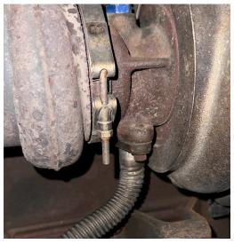
**STEP 10:** Remove the two bolts holding the exhaust hanger from the transmission to assist in aligning the new turbocharger.
