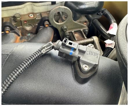
**STEP 3:** Remove oil feed line to turbo and intercooler pipe from the cold side of the turbo. When removing the Intercooler pipe be mindful of not damaging the boot.
