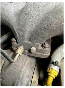
**STEP 7:** With the turbocharger removed you will notice two small alignment pins on the factory cast elbow. If you are installing a stock turbo you will keep the pins in the elbow, if you are installing a Phatshaft turbo you will need to remove the pins in the elbow with pliers.
