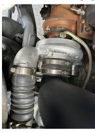
**STEP 4:** Remove the V-band clamp connecting the factory cast elbow to the turbine housing on the exhaust side of the turbo. Loosen the second clamp connecting the down pipe to factory cast elbow so it can be rotated. (2004.5-2007 trucks disconnect the air control valve plug from the factory harness).
