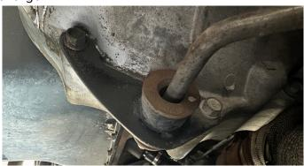
**STEP 11:** Lower the replacement turbo letting it rest on the frame (be sure not to kink or bend the oil drain). Install the studs back into the manifold and turbine housing for the replacement turbo. Line up the turbo to manifold gasket using the studs on the turbo. Lift the turbo to the manifold flange lining the studs up with the holes. Hand tighten the nuts onto the studs to hold turbo in place and start tightening all four nuts to seal the turbo to the manifold.
