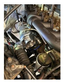
**STEP 12:** Reconnect exhaust elbow to the turbine housing of the turbo along with the intercooler pipe and boot on the front side of the turbo. Reinstall the air intake and reconnect the air flow sensor. Install the oil feed line to the factory fitting you swapped over from the previous unit leaving it loose for now.
